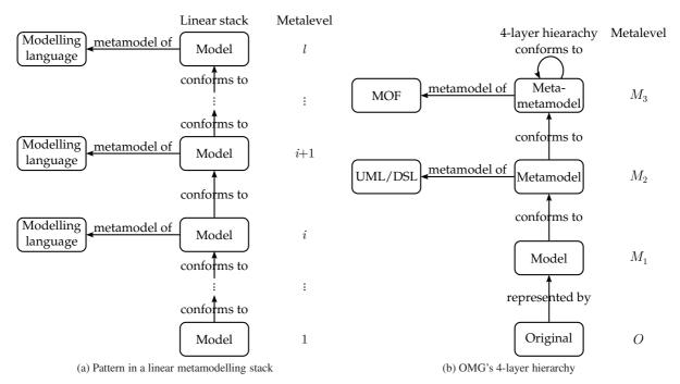
Figure 1. Linear metamodelling stack
